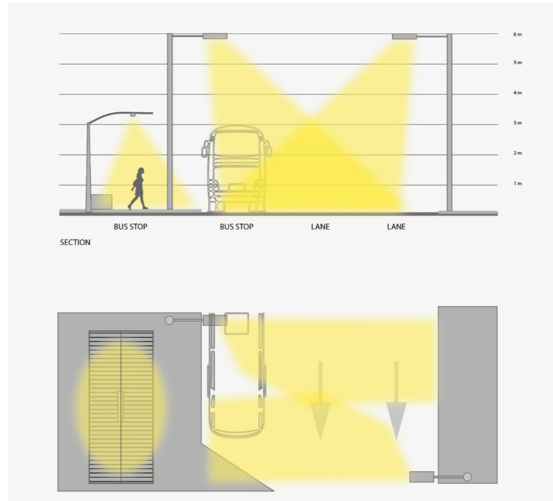
Figure 38: Bus stop typical lighting arrangement
